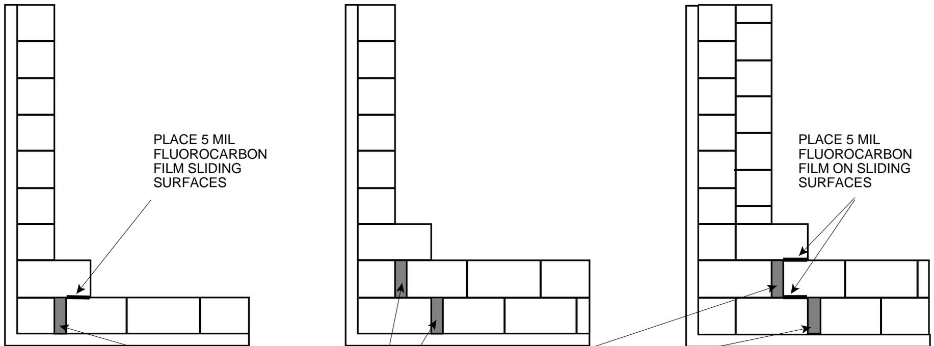
THICKNESS OF COMPRESSIBLE JOINT MUST BE CALCULATED TO BE ADEQUATE IN SIZE SO THAT EXPANSION FORCES IN COMPRESSING DO NOT EXCEED 50% OF THE JOINTWIDTH.
